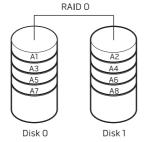
RAID 0 uses the full storage capacities of both drives. For example, two 2 GB hard drives combine to provide 4 GB of hard drive space on which to store data.
